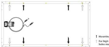
Mounting holes for normal installation For high wind and snow-loads, these mounting holes must also be used
